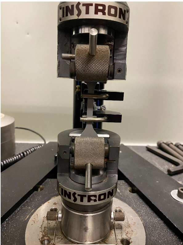
Figure 4 Images of test sample performing durability load / elongation test
